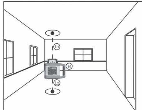
The **SIRIUS 1 HV** is equipped with a self-levelling feature and levels out tilted positioning of the unit by up to 5° in each direction.
